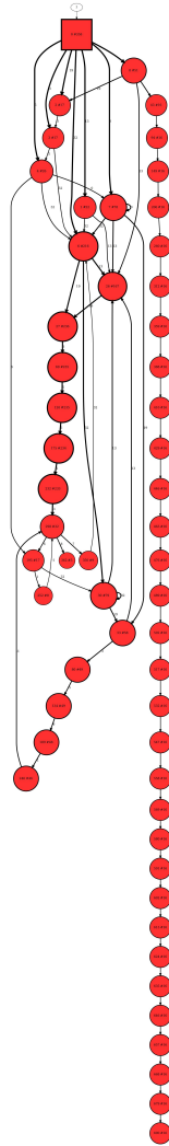
Figure 5.7: The state machine generated for experiment 3. Used initial set of traces S_1 with an abstraction function that uses both input and output traces. Spdfa heuristics are applied.
